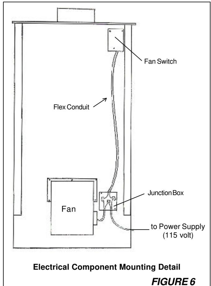
**NOTE:** The fan switch is provided with 3 adjustable pointers. The left pointer (fan off) should be set at 120. The center pointer (fan on) should be set at 150. The right-most pointer is not important for this installation.
